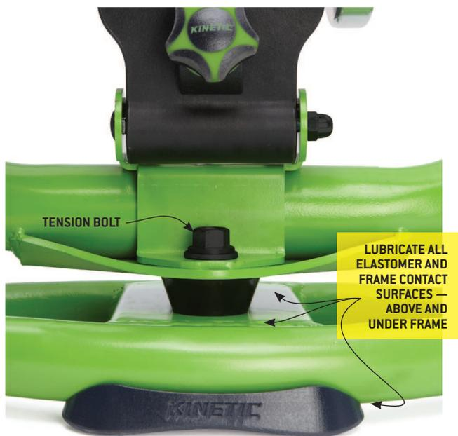
**TIP:** If you partially thread out the tension bolts, you can create a bit of space in the elastomers and the trainer frame, making it easier to get lubricant directly on the contact surfaces without completely disassembling frame.
